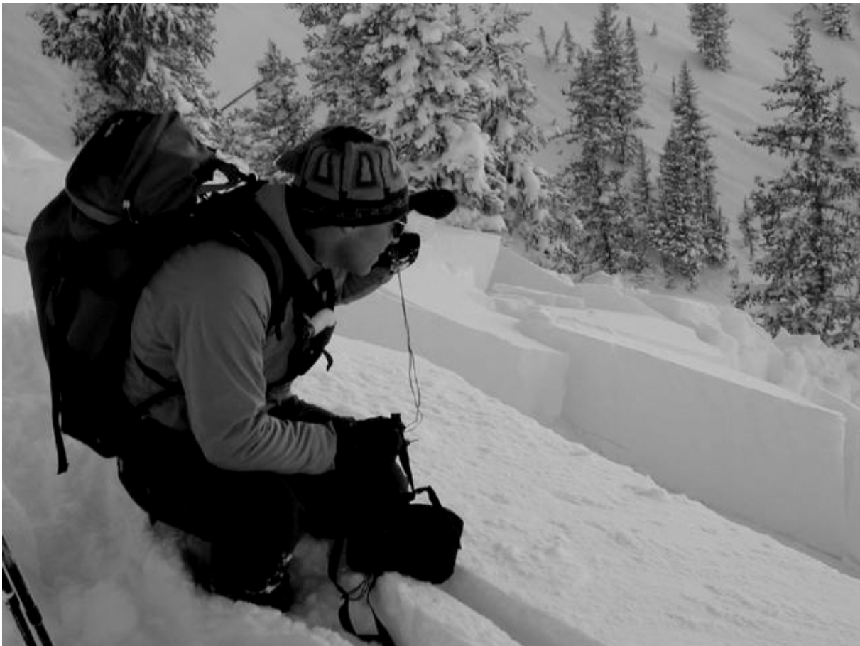
Forest Service Utah Avalanche Center Director, Bruce Tremper, measures the slope steepness of a recent human triggered avalanche in Cardiff Fork. Slope steepness is an extremely critical parameter as just a couple degrees can be the difference between triggering an avalanche and not triggering one. This was a typical avalanche for the season, deep, wide and easily-triggered.
